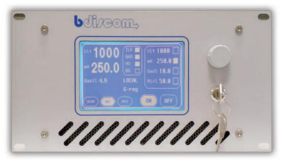
Bdiscom power supply for DC sputter processes. 500 Watt F.S.
